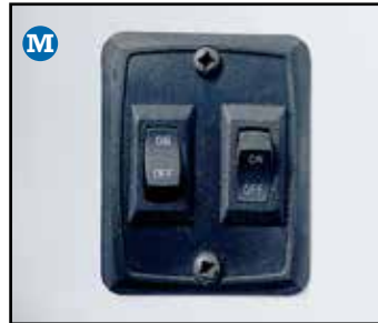
12V Water Pump power switch — left switch is dome light & right switch is water pump.
