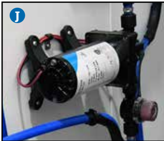
12 Volt Water Pump must be "ON" when using the On-Board Fresh Water Tank
